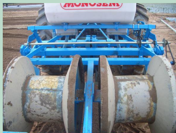
Figure 11: 'Monosem' fertilizer applicator mounted on the ridger.
