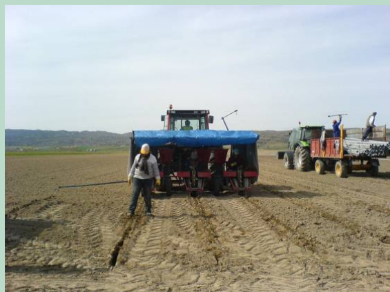
Figure 27: Seeding and application of Multicote™ Agri
