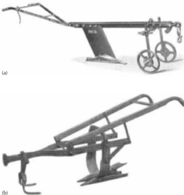
Fig. 2.14 Two designs of horse-drawn implements used during beet harvesting in the UK, c. 1931, (a) for loosening the soil around the plants to make pulling out the roots easier, and (b) for lifting sugar beet roots directly from the soil. © DEFRA/The Stationery Office.
