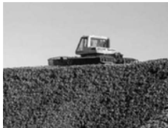
Fig. 15.5 Levelling piles soon after harvest reduces surface area and channelling of air within the pile (American Crystal Sugar Co.).
