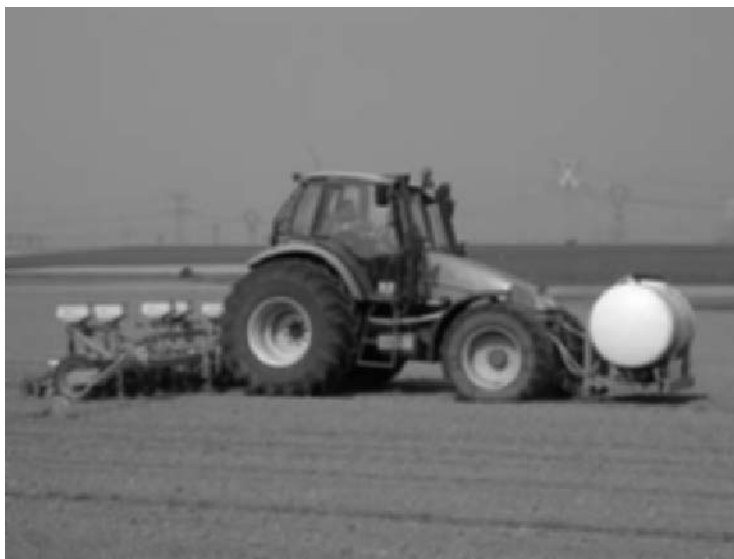
Fig. 8.7 Sowing sugar beet with placed liquid nitrogen fertilizer.
