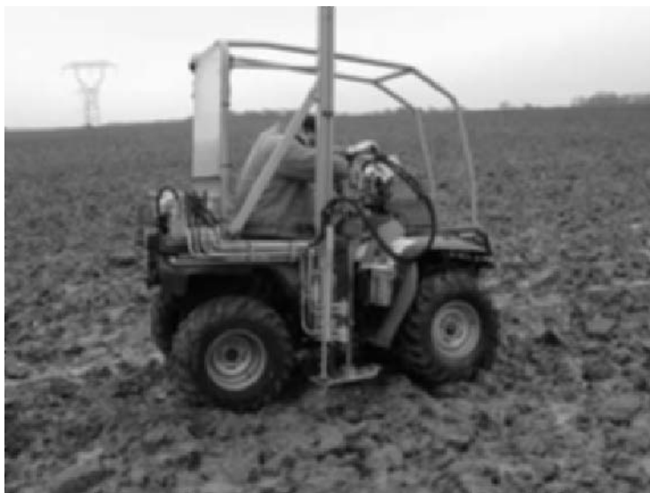
Fig. 8.13 Mechanized collection of soil samples to about 1 m deep prior to sugar beet.
