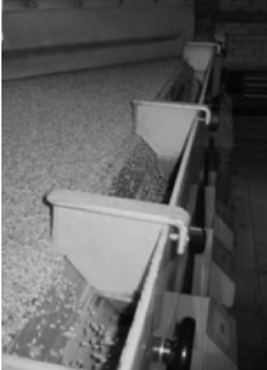
Fig. 5.17 Gravity table for the selection of clusters with well-formed seeds.
