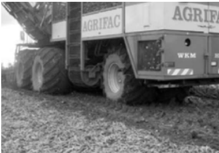
Fig. 6.7 Competitive sugar beet production requires an efficient harvest technique. However, the heavy sugar beet harvesters used today often cause permanent compaction damage to the subsoil, even though damage to the plough layer may be kept within acceptable limits by the use of wide tyres (Photograph: Robert Olsson, SBU, Sweden).
