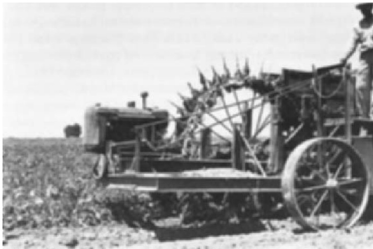
Fig. 2.15 Marbeet one-row sugar beet harvester in California (c. 1942); sugar beet plants are lifted before topping.
