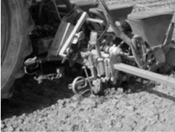
Fig. 8.8 Liquid nitrogen fertilizer being injected through a coulter a few cm to the side and below the seed.
