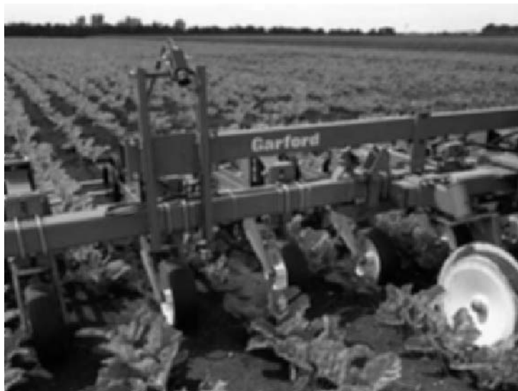
Fig. 14.7 A tractor hoe fitted with vision guidance system (© British Sugar Beet Review).
