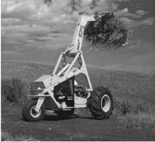
Fig. 7.4 Tricycle loaders. Source: Bell Equipment Pty Ltd, South Africa.
