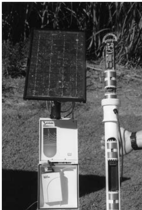
Fig. 5.16 EnviroSCAN soil moisture probe and data logger. Source: Sentek Pty Ltd, Australia.
