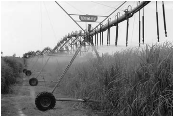
Fig. 5.10 Centre pivot irrigator with low-pressure nozzles on drop tubes. Source: Valmont Irrigation, USA.
